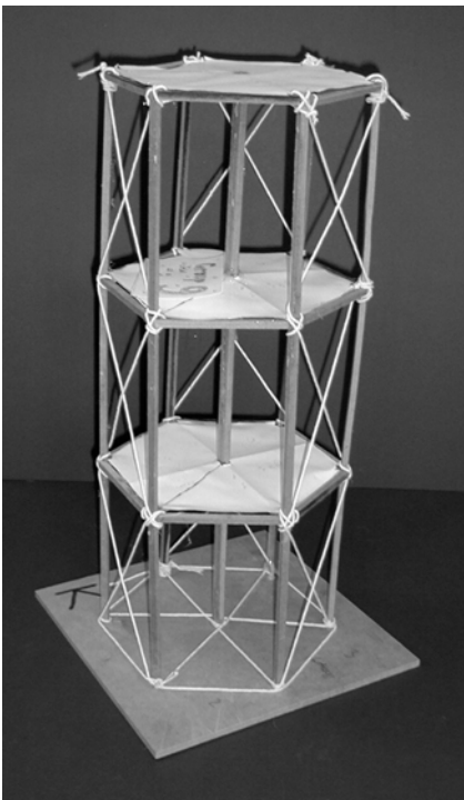
Figure 4: On this hexagonal model, only 3 of the 6 faces in each storey have material between the bottom of one floor and the top of the floor below, so that leaves half the perimeter clear of material.
