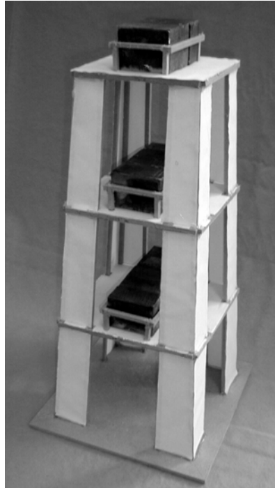
Figure 3: On each face of this model only half the perimeter of each storey has material between the bottom of the floor above and the top of the floor below
